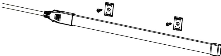
1 / **CONECTORES ENTRE TIRAS** : PEGAR LAS CONTERAS CON COLA DE PVC. DEJAR SECAR DURANTE 30 MINUTOS / **ZWISCHENSTECKTEILE**: DIE ABSCHLUSSKAPPEN MIT PVC-KLEBER VERSIEGELN. 30 MINUTEN TROCKNEN LASSEN / **CONNETTORI INTERBAN-DA**: SIGILLARE LE PLACCHE CON COLLA PVC. LASCIAR ASCIUGARE PER 30 MINUTI
